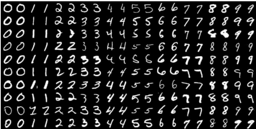
Figure D.10: Reconstructions for the MNIST dataset. Odd columns represent real data and even columns correspond to their reconstructions. The real label is used to sort the column pairs.
