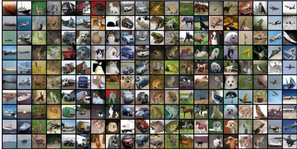
Figure D.7: Generated images for the CIFAR-10 dataset. Every two columns we set a different value for the categorical latent variable y . i.e. the samples shown correspond to a different conditional latent space z \sim p(z|y) .
